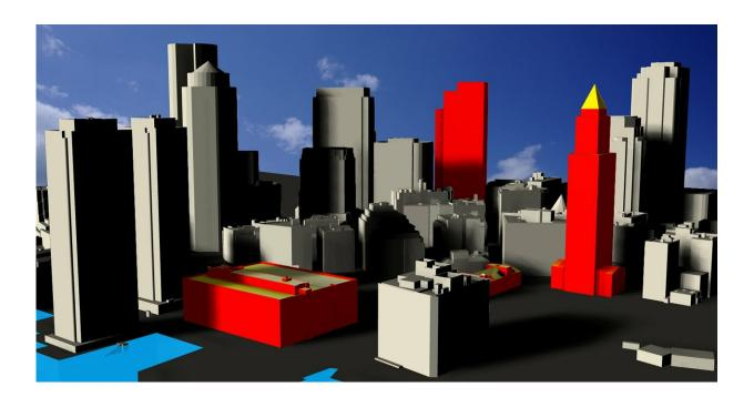
The work carried out at the PVMD group can be used to calculate the solar photovoltaic energy potential of buildings in complex urban landscapes. The image shows results of the model applied to selected façades and roofs of buildings in the city of Boston, Mass. Roofs are painted with brighter colors than façades which indicates a higher energy potential. Base 3D model by Boston Planning & Development Agency is licensed under CC BY 3.0. Credit: Boston Planning & Development Agency
