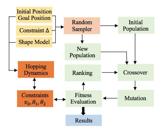
Schematic of the optimized path planner using Evolutionary Algorithm. Credit: Kalita & Thangavelautham.
