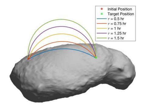
Hopping Trajectories from initial location to a target location on the surface of Itokawa. Credit: Kalita & Thangavelautham.
