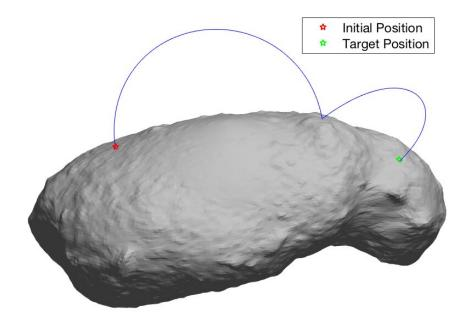
Optimal trajectory generated by the path planner to reach a target location. Credit: Kalita & Thangavelautham.
