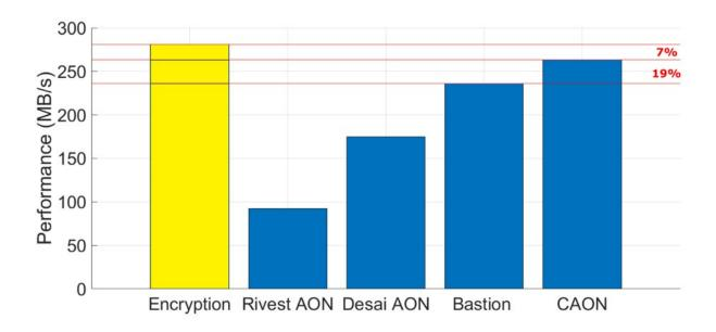
A performance benchmark, comparison between CAON and other techniques, simple encryption (AES-NI in CTR mode, yellow) is used as the baseline. Credit: Kapusta, Memmi & Rambaud.
