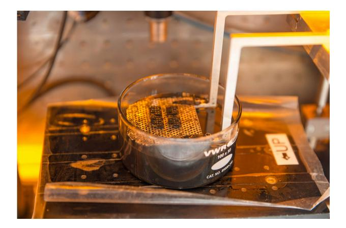
A series of mechanical logic gates are 3D-printed using the Large Area Projection Microstereolithography (LAPµSL) method. Credit: Lawrence Livermore National Laboratory
