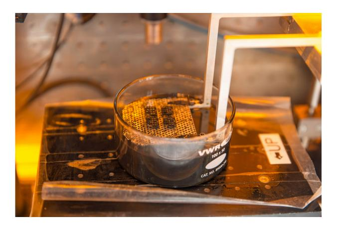
A series of mechanical logic gates are 3D-printed using the Large Area Projection Microstereolithography (LAPμSL) method. Credit: Lawrence Livermore National Laboratory
