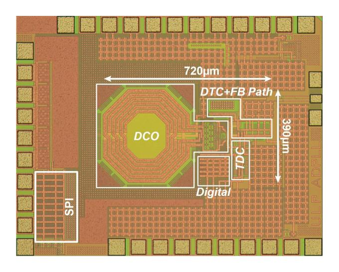
The proposed fractional-N DPLL occupies an area of 0.25 mm<sup>2</sup> in 65-nanometer CMOS. Credit: Kenichi Okada
