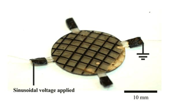
An initially flat thin circular sheet of elastomer morphs into a dome shape based on which sets of electrodes are turned on or off Credit: the Clarke Lab/Harvard SEAS
