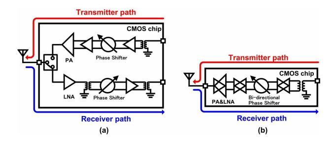
(a) The conventional transceiver structure and (b) the newly proposed bidirectional transceiver structure, which is much more compact. Credit: Atsushi Shirane
