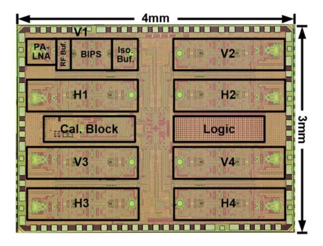
The transceiver consists of a total of four horizontal (H1-4) and four vertical (V1-4) array orientations. Credit: Atsushi Shirane
