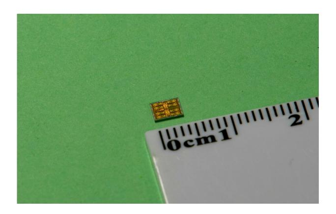
The proposed chip, fabricated in a standard 65-nanometer CMOS process, takes up a total area of just 12 mm<sup>2</sup>. Credit: Atsushi Shirane
