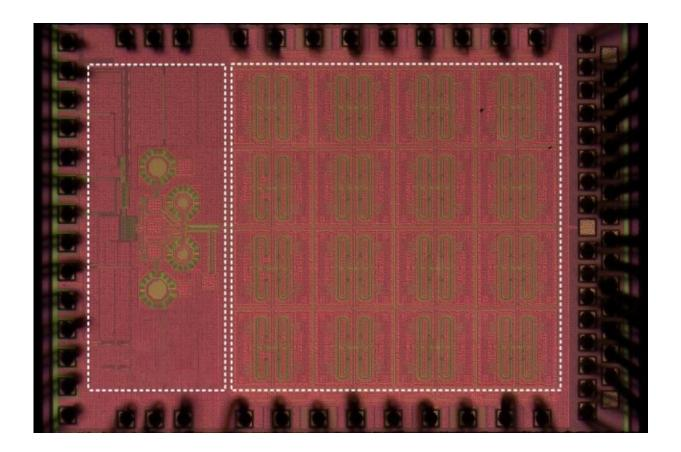
MIT researchers have developed a chip that leverages sub-terahertz wavelengths for object recognition, which could be combined with light-based image sensors to help steer driverless cars through fog. Credit: Massachusetts Institute of Technology
