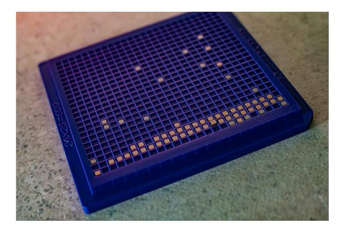
Rice's new design for creating security keys with a physically unclonable function (PUF) proved more reliable, more energy efficient and smaller than previously published PUF technologies. Credit: Jeff Fitlow/Rice University
