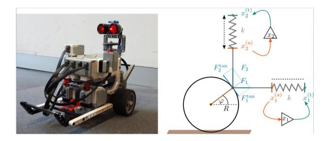
Lego robot and the controller mechanism we used. Credit: Sándor et al.
