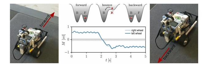
Depicting how the robot changes autonomously the directions of locomotion when hitting a wall. Credit: Sándor et al.
