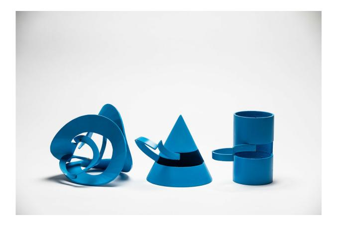
This image shows how developable mechanisms reside in the surface of an object. Credit: BYU
