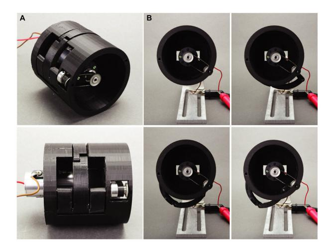
Motorized cylindrical-developable mechanism. A motorized, fully revolving linkage emerging from a cylinder that results in a walking motion. Credit: Nelson et al., *Sci. Robot.* 4, eaau5171 (2019)
