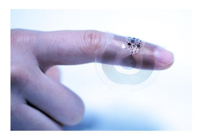
Weighing as much as a raindrop, the chest sensor can wirelessly monitor heart rate, breathing rate, and temperature. Credit: John A. Rogers/Northwestern University
