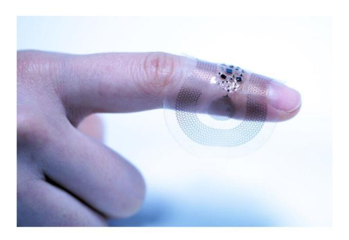
Weighing as much as a raindrop, the chest sensor can wirelessly monitor heart rate, breathing rate, and temperature. Credit: John A. Rogers/Northwestern University
