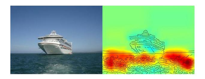
The heatmap shows quite clearly that the algorithm makes its ship/not ship decision on the basis of pixels representing water and not on the basis of pixels representing the ship. Credit: *Nature Communications*, CC BY Lizenz
