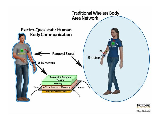
A device keeps communication signals within the body, so that no one can hack into medical equipment such as pacemakers. Credit: Purdue University image/Debayan Das
