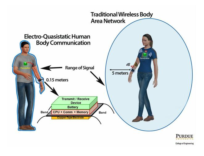
A device keeps communication signals within the body, so that no one can hack into medical equipment such as pacemakers. Credit: Purdue University image/Debayan Das
