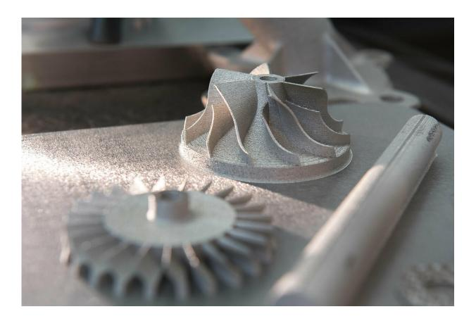
Titanium parts printed from powder and a laser provide researchers with highstrength, heat-resistant examples of the future of additive manufacturing. Credit: U.S. Army photo by David McNally
