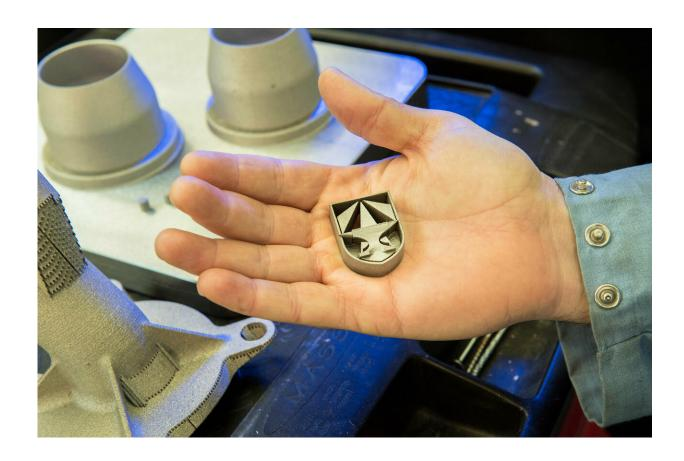
Using advanced additive manufacturing techniques, Army scientists work with an Air Force-invented steel alloy to print intricate geometries with ultra-high-strength. This sample, created using a technique called powder bed fusion, is the symbol of the newly formed Army Futures Command. The steel is 50 percent stronger than what is commercially available. Credit: US Army photo by David McNally
