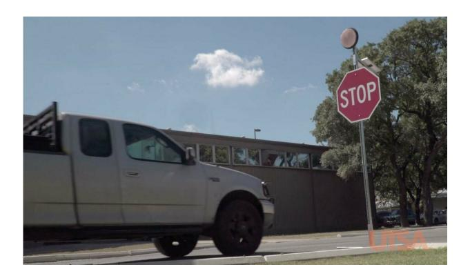
The next-generation stop sign uses a multi-pixel passive infrared sensor that detects a vehicle as it approaches an intersection. Once the vehicle is within the sensing range, a signal beacon triggers the stop sign's flashing system. Credit: UTSA
