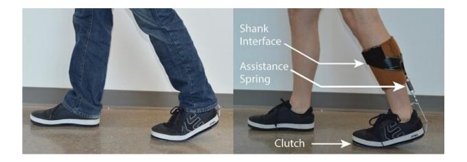
The new ankle exoskeleton design integrates into the shoe and under clothing. Credit: Matthew Yandell
