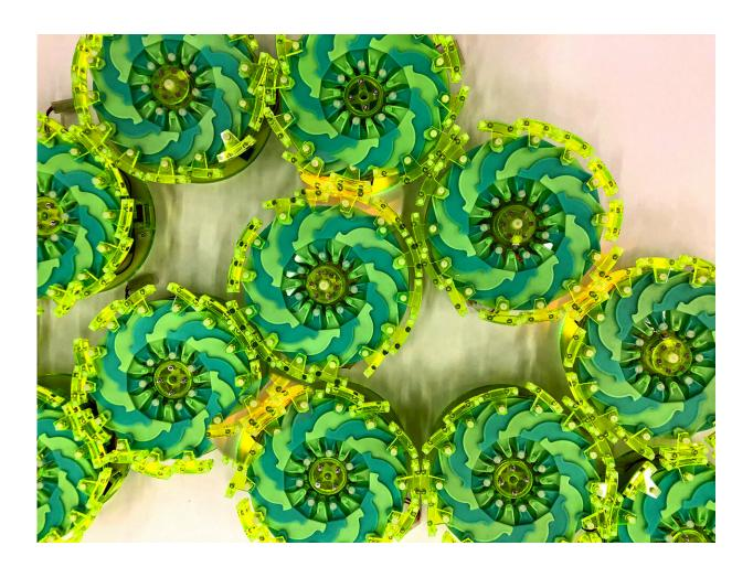
Researchers from MIT and elsewhere have developed computationally simple robots that connect in large groups to move around, transport objects, and complete other tasks. Credit: Felice Frankel
