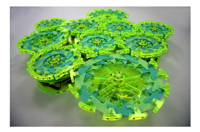
Particle robots are composed of loosely coupled components, or particles, that lack an individual identity or addressable position. They are capable of only a simple motion -- expansion and contraction. However, when a group of particles is coordinated to move as a collective, interesting behavior is observed. Even in amorphous configurations, particle robots exploit statistical mechanics phenomena to produce locomotion. Credit: Shuguang Li/Columbia Engineering
