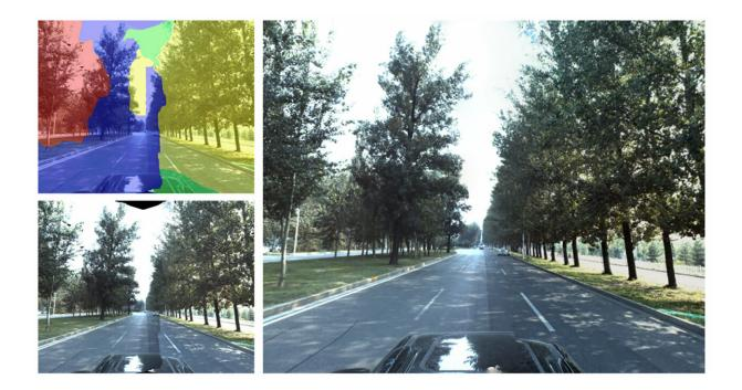
The synthesis of new backgrounds. A "stitching" method was used to make a complete image (left). The final view was synthesized after post-processing processes, like hole filling and color blending. Credit: Li et al., Sci. Robot. 4, eaaw0863 (2019)
