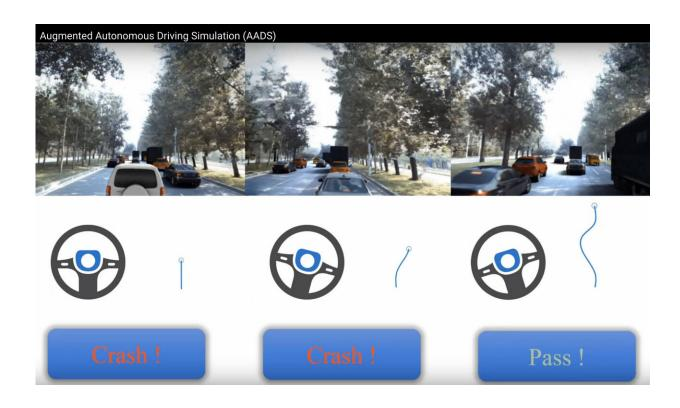
The Augmented Autonomous Driving Simulation (AADS) system combines photos, videos, and lidar point clouds for realistic scene rendering with real-world trajectory data that can be used to predict the driving behavior and future positions of other vehicles or pedestrians on the road. Credit: Li et. Al, 2019
