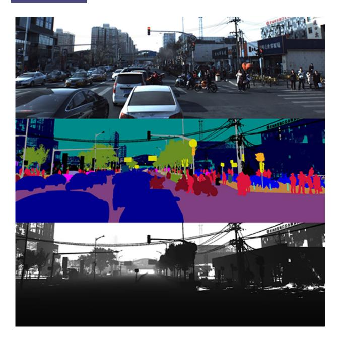
The dataset produced by the AADS system, including RGB images (top), annotations of different objects (middle), and a point cloud (a set of data points in space). Credit: Li et al., Sci. Robot. 4, eaaw0863 (2019)
