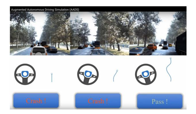
The Augmented Autonomous Driving Simulation (AADS) system combines photos, videos, and lidar point clouds for realistic scene rendering with realworld trajectory data that can be used to predict the driving behavior and future positions of other vehicles or pedestrians on the road. Credit: Li et. Al, 2019
