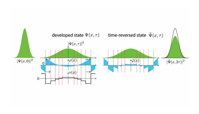
Image shows a time reversal procedure for a spreading wave packet that represents a quantum particle. The reversed state freely evolves into the original squeezed state, which is recovered with some precision -- in this case, 85 percent. (Image by Argonne National Laboratory. Credit: Argonne National Laboratory
