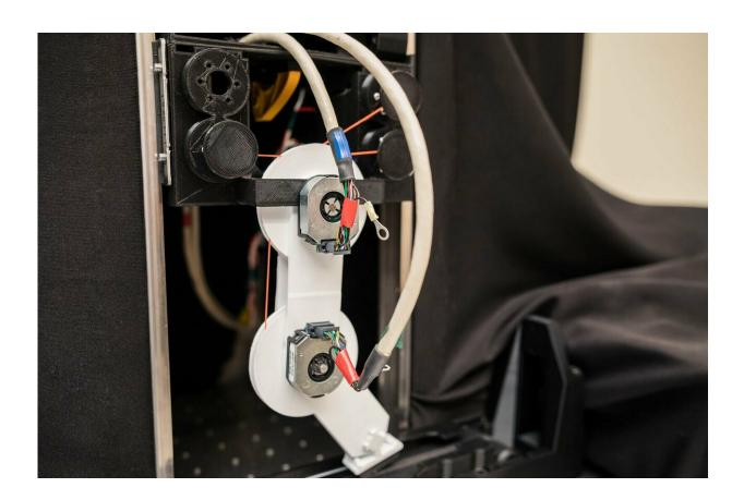
A team of researchers at the USC Viterbi School of Engineering believe they have become the first to create an AI-controlled robotic limb driven by animallike tendons that can even be tripped up and then recover within the time of the next footfall, a task for which the robot was never explicitly programmed to do. Credit: Matthew Lin
