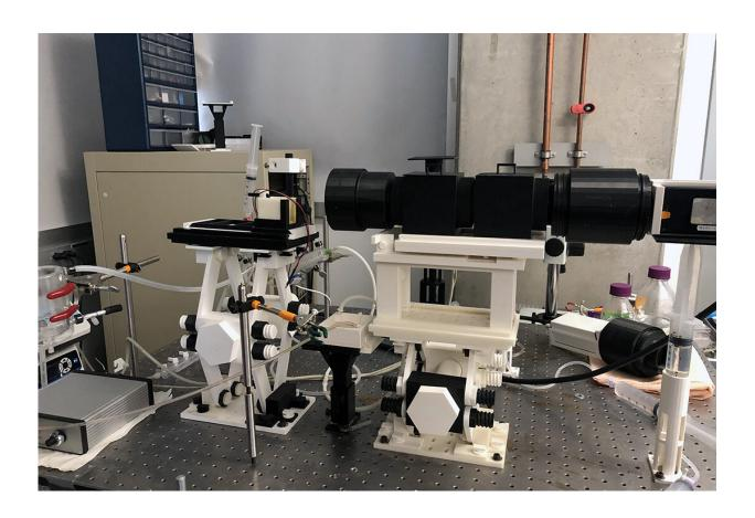
Researchers can download specific pieces of a mapping system they want to replicate or the entire system which supports specialized optical equipment including cameras, lenses and mirrors. Credit: George Washington University
