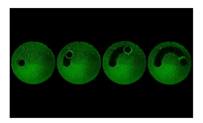
With a precise, controlled movement, microrobots cleared a glass plate of a biofilm, as shown in this time-lapse image. Credit: Geelsu Hwang and Edward Steager
