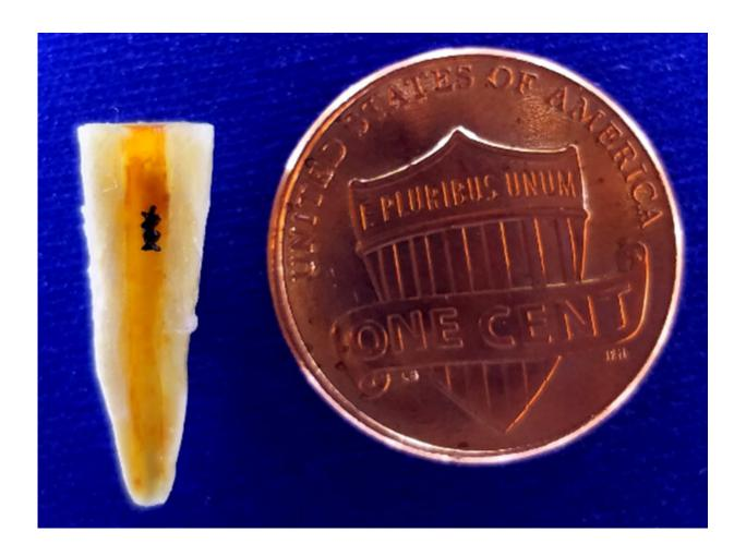
3-D molded helicoidal CARs can be magnetically actuated through the canal of the tooth, another common location of dental biofilm formation. Credit: Hwang et al., Sci. Robot. 4, eaaw2388 (2019)
