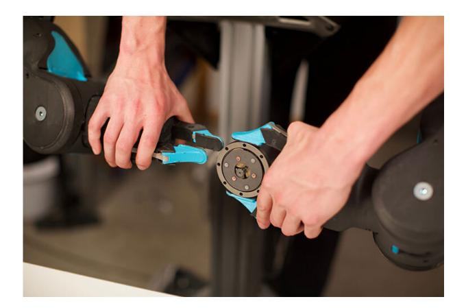
Blue the robot's durable, plastic parts and high-performance motors total less than \$5,000 to manufacture and assemble. Here its grippers are shown holding a gear set. Credit: Philip Downey
