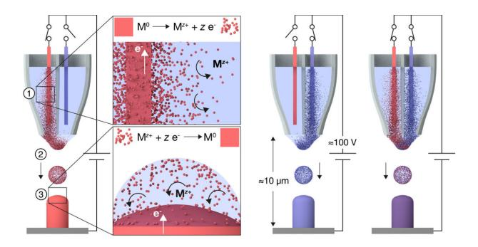
Working principle of 3D printing with metal ions. By applying appropriate voltages one can print, for instance, copper (left), silver (centre) or both metals at the same time (right). Credit: Alain Reiser / ETH Zurich
