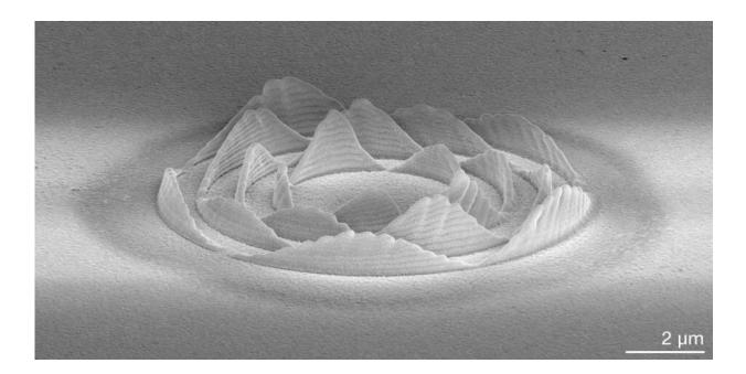
Copper structure printed layer by layer with a spatial resolution of around 200 nanometres. Credit: Alain Reiser / ETH Zurich
