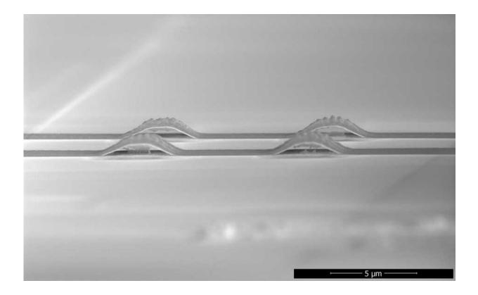
These silver stripes with arched bridges were realized with the help of a supporting structure made of copper, which was subsequently etched away. Credit: Alain Reiser / ETH Zurich
