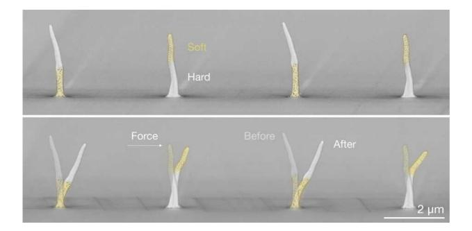
Silver nano-pillars: by etching copper away from the sections with a silvercopper alloy (yellow), their porosity was increased. In those places the material is less stable, which becomes visible when a force is applied (bottom figure). Credit: Alain Reiser / ETH Zurich
