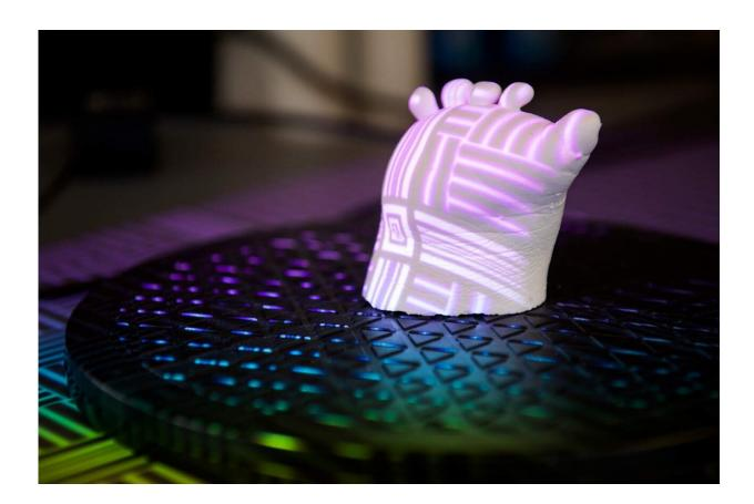
The mold of local teen Josie Fraticelli's hand that was scanned during the development of a personalized prosthetic. Photo by Logan Wallace. Credit: Virginia Tech
