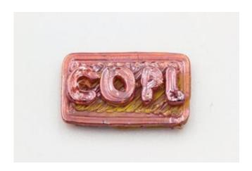
Researchers demonstrated 3D printing of chalcogenide glass, which can be used to make optical components that operate at mid-infrared wavelengths. This 3D printed glass sample is 14 millimeters long. Credit: Steeve Morency, Université Laval
