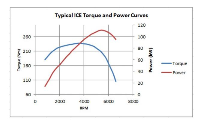
Power and torque characteristics of a typical internal combustion engine. Credit: Victor Barreto
