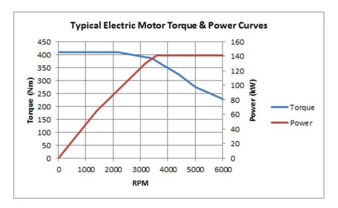
Power and torque characteristics of a typical electric motor. Credit: Victor Barreto
