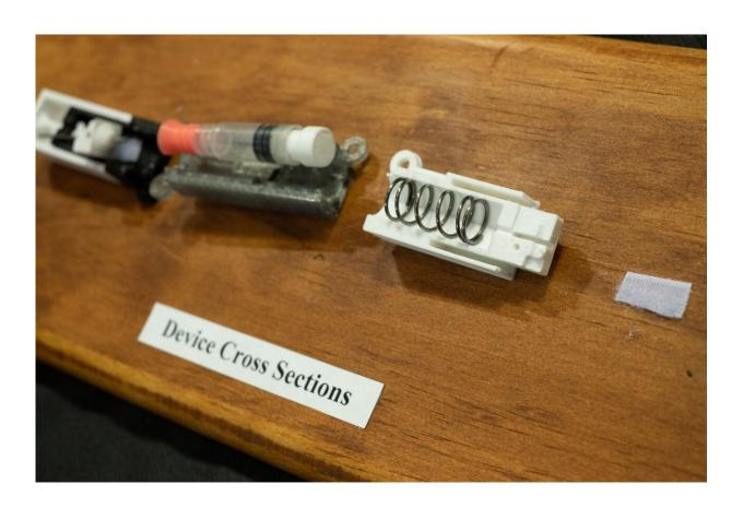
A breakdown shows the internal mechanism of an epinephrine delivery device prototyped by Rice University engineering students. Credit: Jeff Fitlow/Rice
