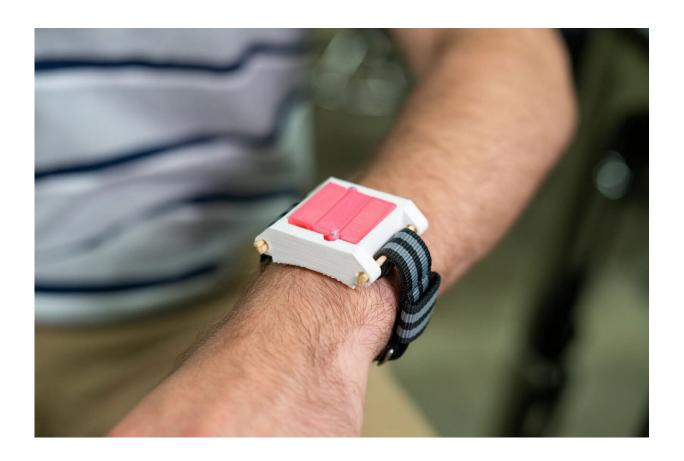
The goal of a team of Rice University students is to create a wearable epinephrine delivery device that people prone to allergic reactions can keep on them and handy at all times. Larger prototypes served as the proof-of-concept that a spring-loaded, trifold device can effectively deliver a full dose of epinephrine. Credit: Brandon Martin/Rice University
