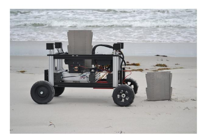
The robot is designed by Wyss Institute researchers to drive interlocking sheet piles into granular soils like sand on a beach. Credit: Wyss Institute at Harvard University
