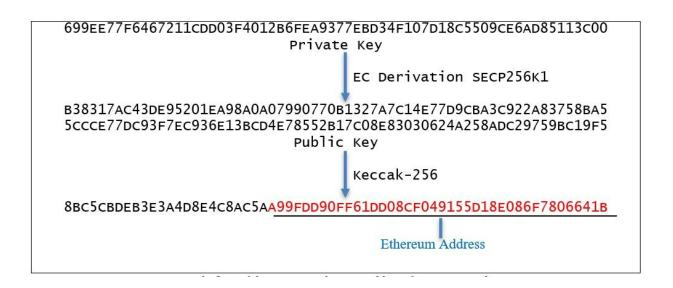
Example flow of deriving an Ethereum address from a private key. Credit: Independent Security Evaluators
