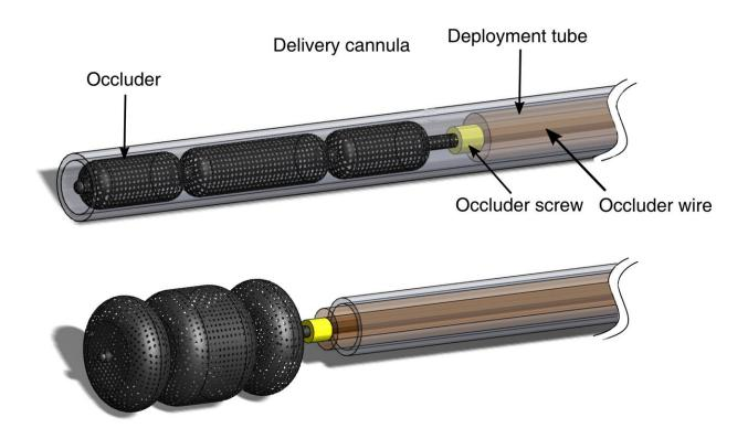
A diagram of the occluder deployment system. Credit: Fagogenis et al., Sci. Robot. 4, eaaw1977 (2019)
