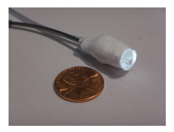
The tip of the catheter comprised a haptic vision sensor made of a millimeterscale camera and LED encased in silicone. Credit: Fagogenis et al., Sci. Robot. 4, eaaw1977 (2019)
