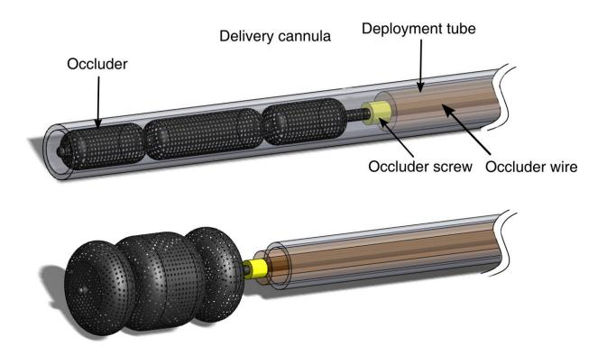
A diagram of the occluder deployment system. Credit: Fagogenis et al., Sci. Robot. 4, eaaw1977 (2019)
