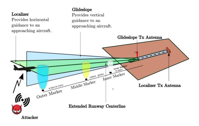
Overview of ILS sub-systems. The ILS consists of three subsystems: i) Localizer, ii) glideslope, and (iii) marker beacons. Credit: Harshad Sathaye, et al.
