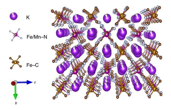
The typical structure of the  $K_xFe_yMn_{1-y}[Fe(CN)_6]_w$ ·zH<sub>2</sub>O in the P21/n space group. Credit: *Nature Energy* (2019). DOI: 10.1038/s41560-019-0388-0
