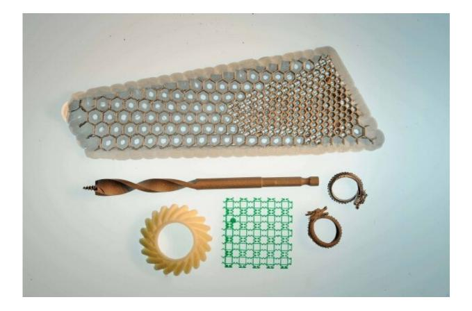
3-D-printed objects related to Professor John Hart's research including: a scale model of an optimized airplane wing core (top); a metal drill bit and two rings (center and right) produced by Desktop Metal, a company Hart co-founded in
