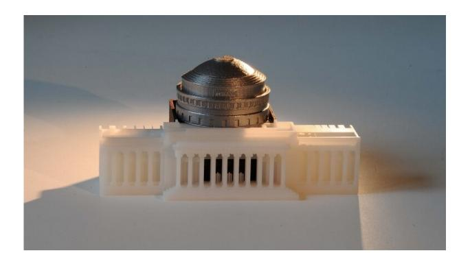
Each component of this three-piece assembly of MIT's Building 10 dome was printed using a different commercial additive manufacturing process. The piece was modeled after an original design by Ely Sachs and Michael Cima after their invention of binder jet printing. Credit: Felice Frankel
