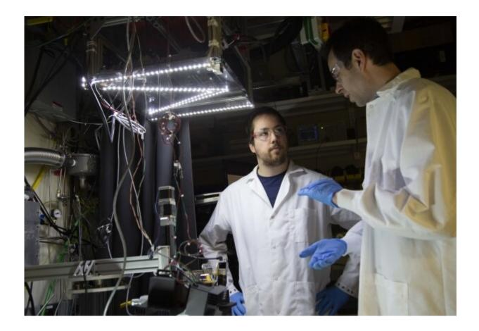
Associate Professor John Hart speaks with graduate student David Griggs in front of his lab's custom-built selective laser melting system. In the system, a laser is precisely scanned over metal powder, melting the powder to form a 3-D part layer by layer. Credit: John Freidah
