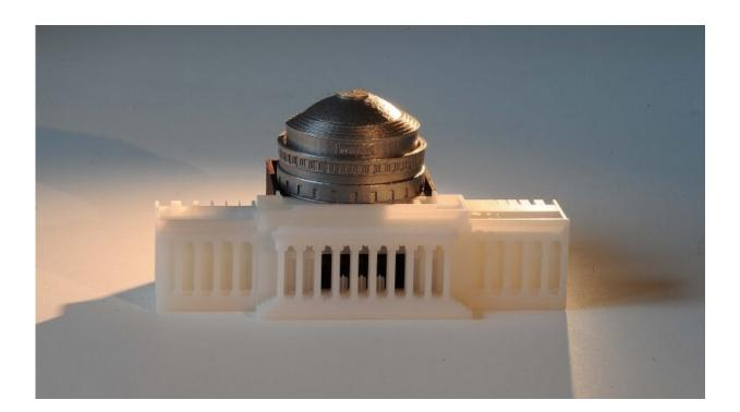
Each component of this three-piece assembly of MIT's Building 10 dome was printed using a different commercial additive manufacturing process. The piece was modeled after an original design by Ely Sachs and Michael Cima after their invention of binder jet printing. Credit: Felice Frankel
