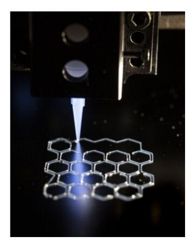
Associate Professor Xuanhe Zhao and PhD candidate Hyunwoo Yuk use 3-D printing technologies to create complex 3-D structures. Here, a polymer scaffold ink is being printed on a silicon wafer to provide structural support for other ink materials with poorer printability during the 3-D printing process. This scaffold ink can be washed away after printing, leaving a complex 3-D structure made of hard-to-print materials. Credit: John Freidah
