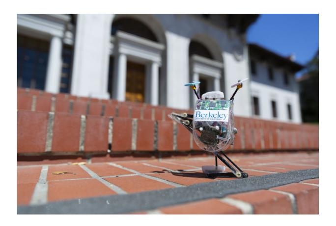
Researchers at the University of California, Berkeley, first unveiled Salto the jumping robot in 2016. Now, they've equipped the robot with a slew of new skills, giving it the ability to bounce in place like a pogo stick and jump through obstacle courses like an agility dog. Salto can even take short jaunts outside, powered by a radio controller. Credit: UC Berkeley photo by Stephen McNally
