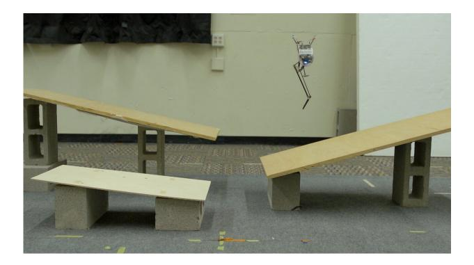
Researchers at the University of California, Berkeley, first unveiled Salto the jumping robot in 2016. Now, they've equipped the robot with a slew of new skills, giving it the ability to bounce in place like a pogo stick and jump through obstacles like an agility dog. Here, it bounces from ramp to ramp in an indoor course. Credit: UC Berkeley photo by Stephen McNally
