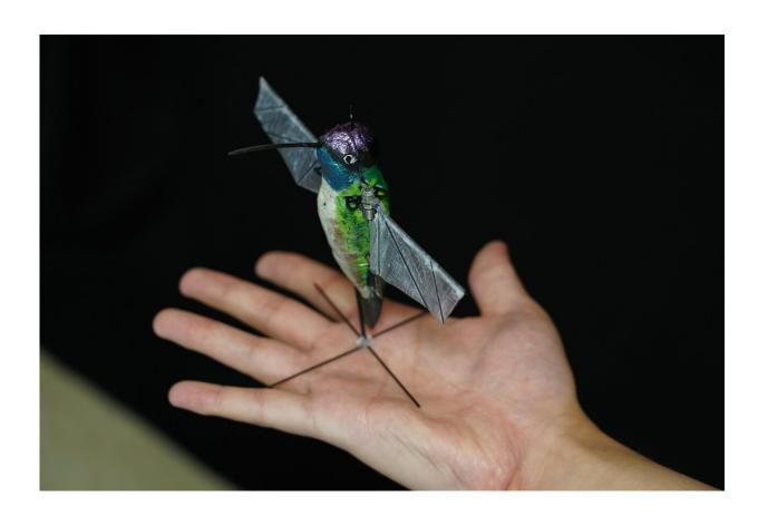
Purdue University researchers are building robotic hummingbirds that learn from computer simulations how to fly like a real hummingbird does. The robot is encased in a decorative shell. Credit: Purdue University photo/Jared Pike
