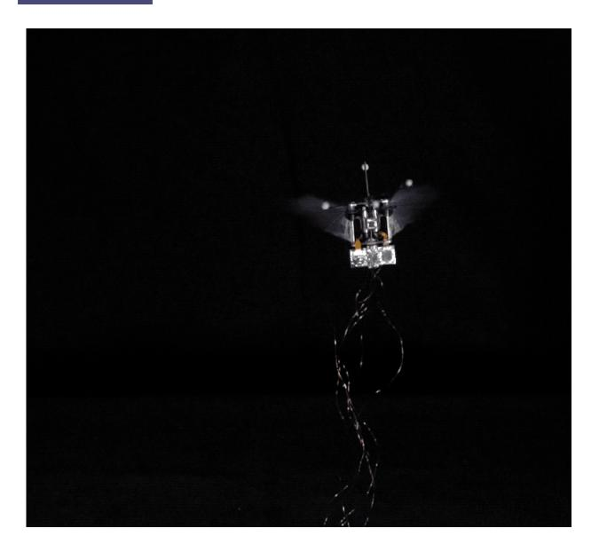
This robotic hummingbird flies on its own while tethered to an energy source, but will soon be powered on batteries. Credit: Purdue University video/Bio-Robotics Lab
