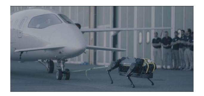
HyQReal has been tested in Genova Airport, in Genoa (Italy), with the support of Piaggio Aerospace. HyQReal was able to pull a small passenger airplane (Piaggio P180 Avanti), 3300 kg weight, 14.4 m long, with a wingspan of 14 m. Credit: IIT-Istituto Italiano di Tecnologia
