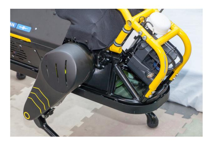
HyQReal is 1,33 m long and 90 cm tall, and its weight is 130kg considering hydraulics and batteries onboard. The robot is protected by an aluminium roll cage and a skin made of Kevlar, glass fiber and plastic. Credit: IIT-Istituto Italiano di Tecnologia
