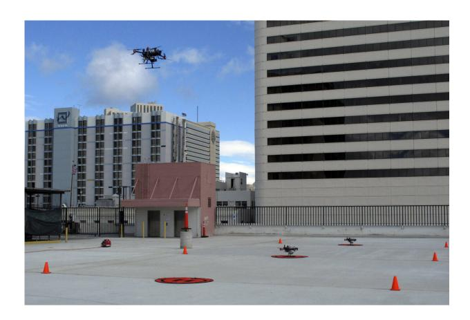
In this Tuesday, May 21, 2019 photo, a drone takes off from the roof of the Cal-Neva casino parking garage in downtown Reno, Nev. as part of a NASA simulation to test emerging technology that someday will be used to manage travel of hundreds of thousands of commercial, unmanned aerial vehicles (UAVs) delivering packages. It marked the first time such tests have been
