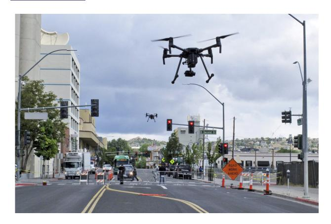
In this May 21, 2019 photo, two drones fly above Lake Street in downtown Reno, Nev., on, as part of a NASA simulation to test emerging technology that someday will be used to manage travel of hundreds of thousands of commercial, unmanned aerial vehicles (UAVs) delivering packages. It marked the first time such tests have been conducted in an urban setting. (AP Photo/Scott Sonner)
