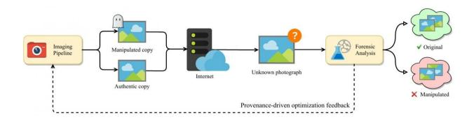
In tests, a prototype pipeline increased the ability to detect manipulation from approximately 45 percent to over 90 percent without sacrificing image quality. Credit: NYU Tandon
