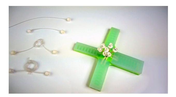
This new, simplified soft robot, powered by pressurized air, replaces multiple control systems with one input, reducing the number, weight and complexity of the components needed to power the device. Credit: Bertoldi Lab/Harvard SEAS
