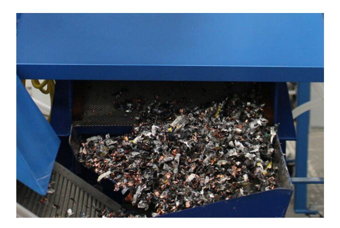
Li-Cycle's demonstration plant in Kingston, Ont safely shreds batteries – the first step in the startup's innovative process for recycling up to 90 per cent of the battery's material. Credit: Li-Cycle
