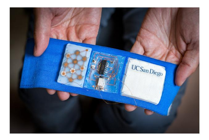
Armband embedded with flexible battery pack (left), stretchable circuit (center), and cooling/heating patch (right). Credit: David Baillot/UC San Diego Jacobs School of Engineering
