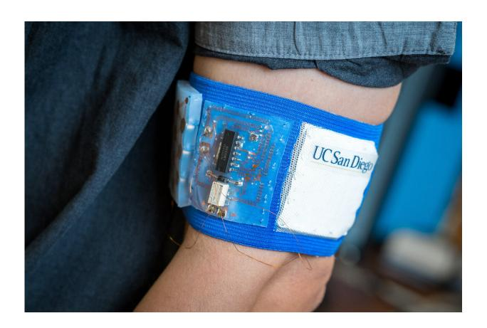
Prototype of the cooling and heating patch embedded in a mesh armband. Credit: David Baillot/UC San Diego Jacobs School of Engineering
