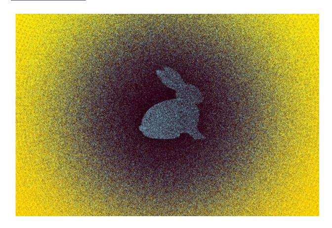
Robots currently attempt to identify objects in a point cloud by comparing a template object — a 3-D dot representation of an object, such as a rabbit — with a point cloud representation of the real world that may contain that object. Credit: Christine Daniloff, MIT
