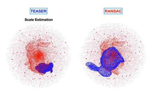
The MIT-developed technique quickly and smoothly matches objects to those hidden in dense point clouds (left), versus existing techniques (right) that produce incorrect, disjointed matches. Credit: Courtesy of the researchers
