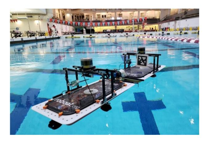
MIT researchers have given their fleet of autonomous "roboats" the ability to automatically target and clasp onto each other — and keep trying if they fail. The roboats are being designed to transport people, collect trash, and self-assemble into floating structures in the canals of Amsterdam. Credit: Massachusetts Institute of Technology
