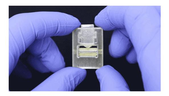
Inkbit's 3-D printer can produce multimaterial objects (like the pinch valve shown above) at high volumes. Credit: Inkbit
