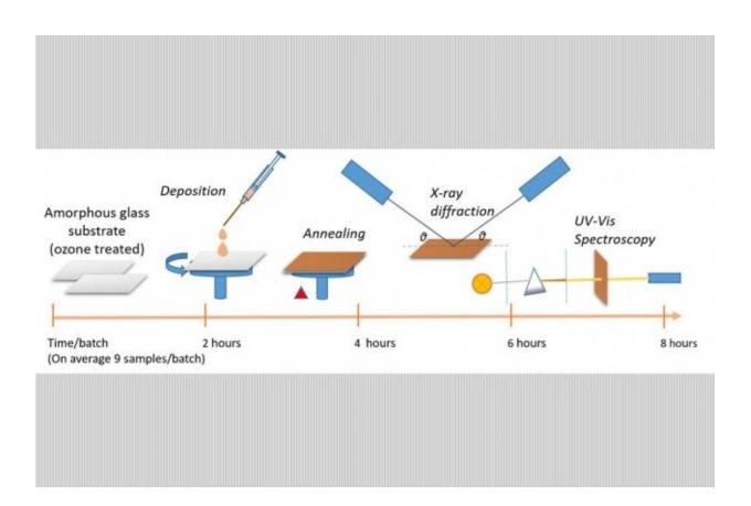
Diagram depicts the sequence of steps used in the new streamlined process to synthesize perovskite-based materials, deposit them on a substrate to create a thin film, and then analyze the film's characteristics using X-ray diffraction and other observational methods. The new process is about ten times faster than previous methods. Credit: Massachusetts Institute of Technology
