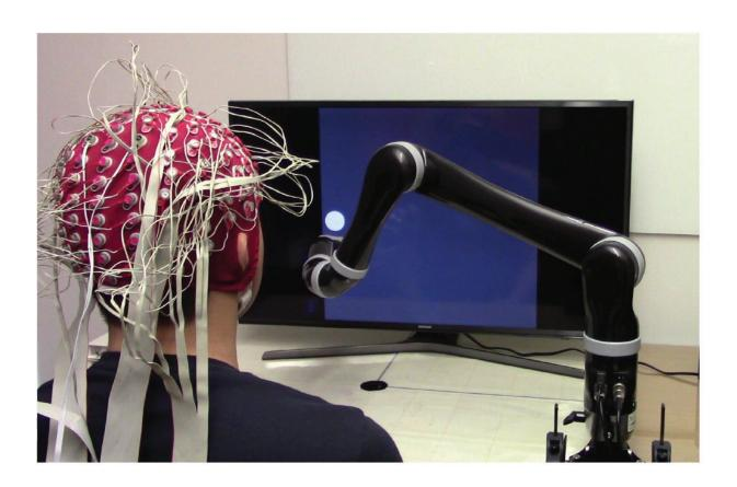
BCI setup using a robotic arm. Users controlled the 2D continuous movement of a robotic arm to track a randomly moving target on a computer screen. Credit: Edelman et al., Sci. Robot. 4, eaaw6844 (2019)
