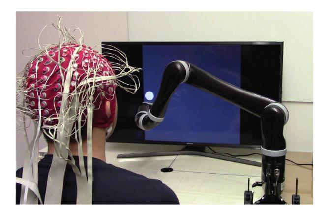
BCI setup using a robotic arm. Users controlled the 2D continuous movement of a robotic arm to track a randomly moving target on a computer screen. Credit: Edelman et al., Sci. Robot. 4, eaaw6844 (2019)
