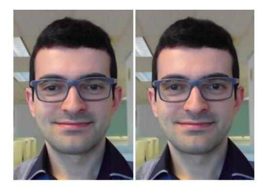
Eye contact correction: in the input frame (left) the user is looking at the screen. In the output frame (right) his gaze is corrected to look into the camera. Credit: Isikdogan, Gerasimow & Michael.
