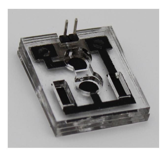
This solid phase bacteria-powered biobattery could be a low-cost power source for the Internet of Disposable Things. Credit: Sean Choi
