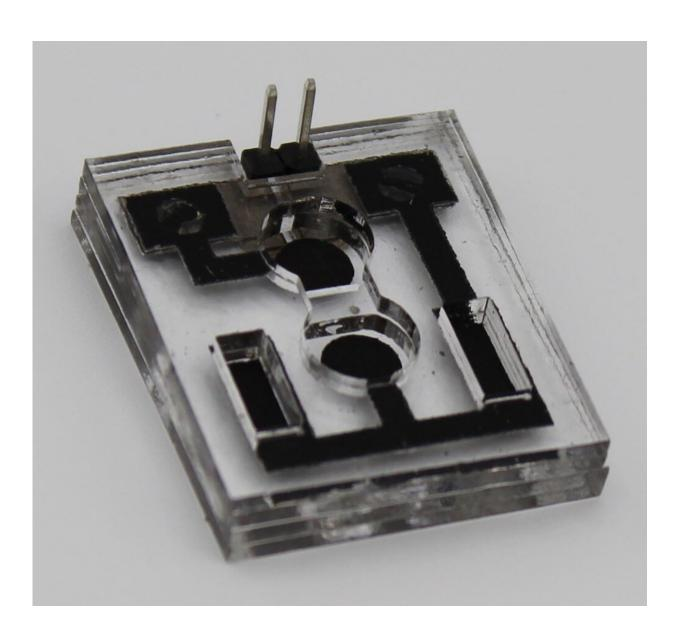
This solid phase bacteria-powered biobattery could be a low-cost power source for the Internet of Disposable Things. Credit: Sean Choi
